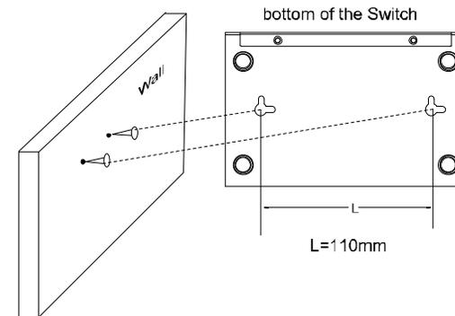
Figure 3-1 Mounting the Switch on a Wall
